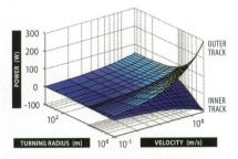
FIGURE 3 Simulation of power consumption of a tracked robot running on dry sand (left) and sandy loam (right).
