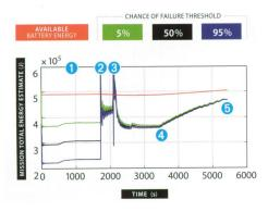
by limiting the power that can be drawn from the battery. This, however, also prevented the robot from following the optimal velocity trajectory and caused it to operate under inefficient conditions. Inefficient operation caused the mission energy requirement predictions to gradually increase. Nevertheless, the mission was completed before another failure was predicted. Figure 6 shows the mission energy requirement predictions during this second simulation.
