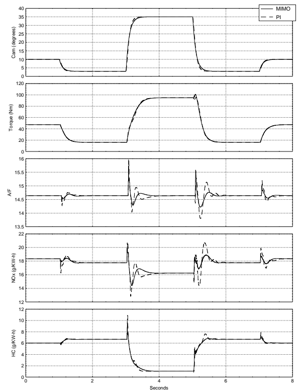
Fig. 15. Simulation response of the multivariable (MIMO) and the decentralized (2 PI loops) control scheme.
