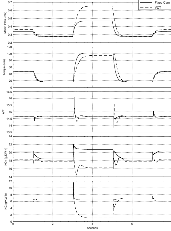
Fig. 16. Simulation response of the conventional ( CAM = 0 ) and the VCT engine.
