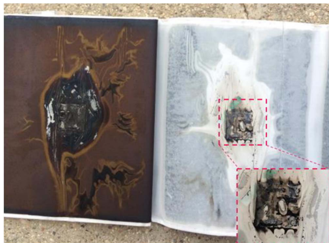
Figure 9. Disassembling result of the battery Ca-An1 after the experiment. Burnt traces can be found around the ISC area.
