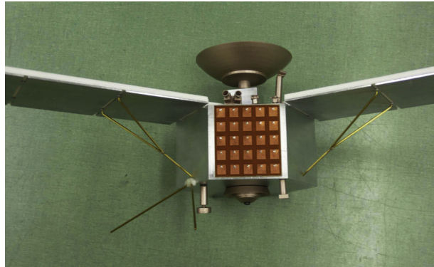
Fig. 13 A functional 22:1 scale model of the A1 antenna mounted on a mockup of the Juno spacecraft for testing
