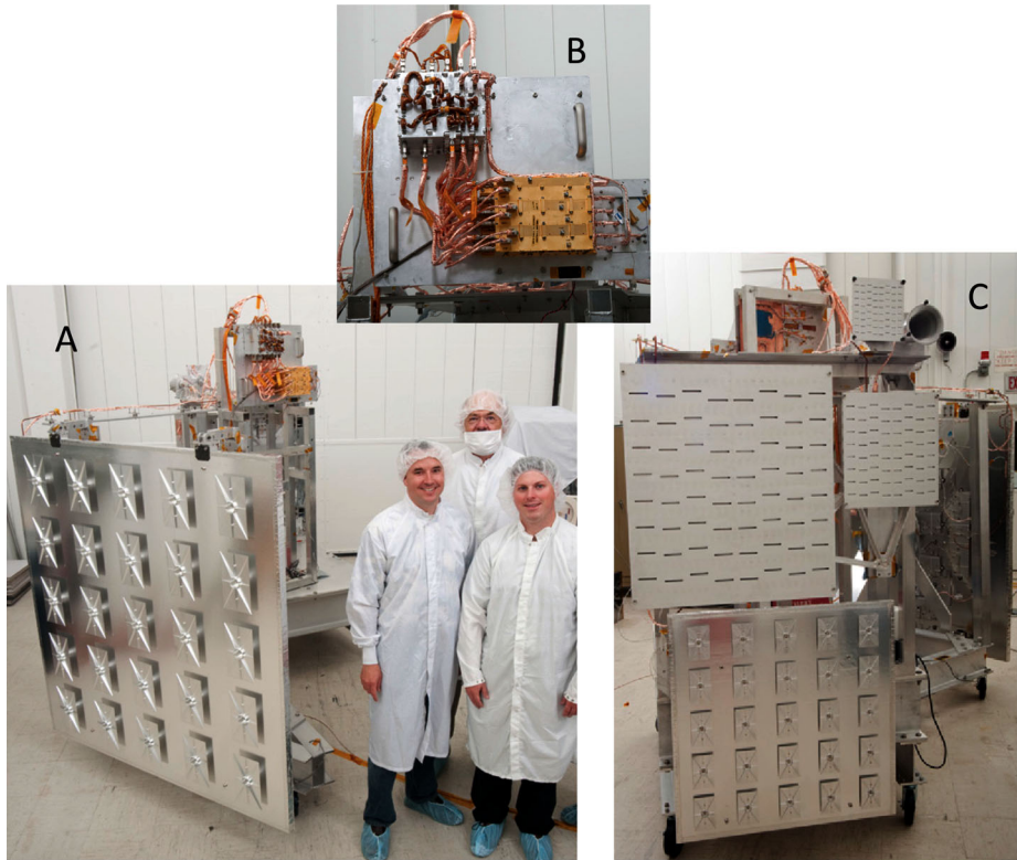
Fig. 7 The MWR Instrument in its flight configuration. The MWR was assembled on a spacecraft mockup frame in May 2010 for end-to-end testing just prior to delivery for spacecraft integration. A. View of the assembled instrument from the A1 antenna side. Left to right, J. Oswald, M. Janssen, and S. Brown. B. The Electronics unit ( upper left ) and Receiver unit ( lower right ). C. View of the assembled instrument from the A2–A6 antenna side
