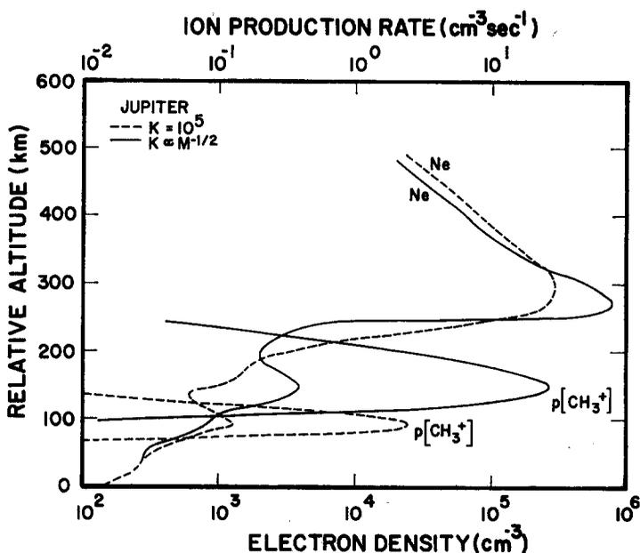
FIG. 2. Jupiter's model ionosphere with  $K = 10^5 \text{ cm}^2 \text{ sec}^{-1}$  and  $K \propto M^{-1/2}$ .  $\text{CH}_3^+$  ion production rates,  $p[\text{CH}_3^+]$ , for the two models are given by the upper scale. Height scale is the same as in Fig. 1.
