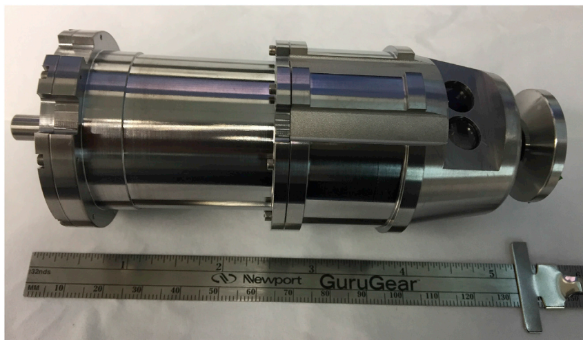
Fig. 9. Saturn probe prototype NFR vacuum micro-vessel with sapphire and diamond windows; this houses a focal plane assembly that accommodates Winston cones with a 5° field-of-view acceptance angle.
