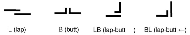
Fig. 6. An example of a joint library for 2-D sheet metal products; LB, a lap-but butt joint with lap on the node with lower index and butt on a node with higher index; BL, the opposite configuration.
