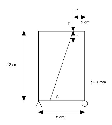
can be maximized, where F is an applied vertical force given as 1 kN per unit length ( i.e. per 1 mm) at the top of the box beam, and d is the vertical deflection at the loading point P. If necessary, use E = 200 Gpa, = 0.3, and = 0 (shear constant), and it is not necessary to consider the possibility of buckling of "beam" elements in compressive axial stress condition, that is, solve the problem under linear elasticity assumption.
