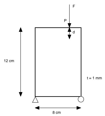
By adding a thin plate, whose thickness is  $t_a$  and the height  $l_a$ , to this box beam for reinforcement while the total volume of the additional reinforced plate is kept to be constant, say  $V_a = t_a * l_a = 120 \text{ mm}^3/\text{mm}$ , find approximately the best location A of the reinforcement so that the local stiffness of the cross section defined by
