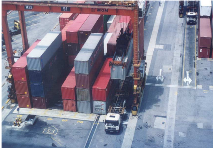
Fig. 2. An RTGC spans the width of a block with seven rows of spaces between its two legs. Six of these rows are used for container storage, the seventh (rightmost in the figure, a parked truck is in the row) is for truck passing.
