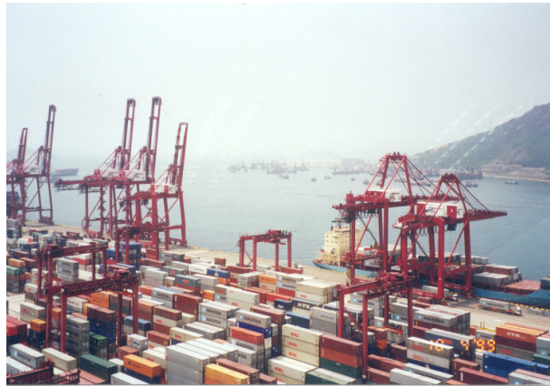
Figure 4: Containers in temporary storage at the SY. At water's edge, see QCs unloading ICs from, and loading ECs into, vessels. In SYs see YCs that store and retrieve containers from storage.
