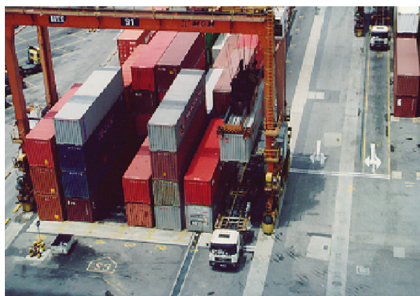
Figure 5: Six rows of stored containers and seventh (rightmost) row used as a lane for truck passage in a storage block. You can see the YC lowering a container retrieved from storage onto an IT.
