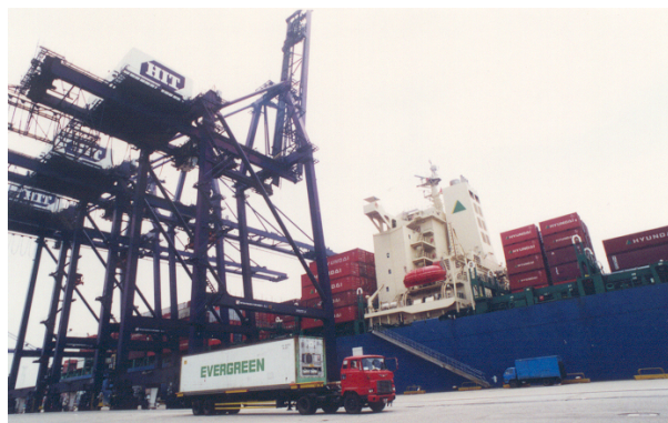
Figure 3: A docked container vessel and QCs unloading inbound containers (ICs) from it and loading outbound containers into it. Also see an IT (that transports containers between the berth and the SY) loaded with an IC that it is taking to the SY.
