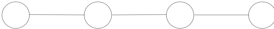
Figure 10.28: This network is not a star, as it has two nodes with degree \geq 2 .
