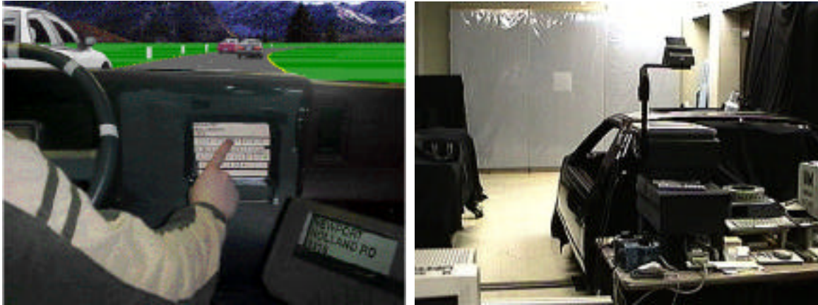
FIGURE 2 Sample scene (left) and setup (right) of the second-generation simulator.
