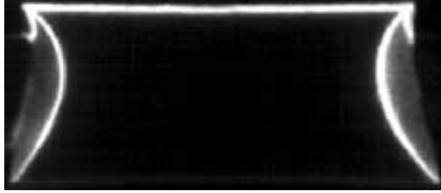
Figure 4. A sample image of a liquid slug. A vertical laser sheet is cast through the tube axis from the right upper side. The left meniscus is illuminated by the same laser sheet redirected by a dielectric mirror.
