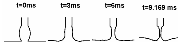
(c) Positive coefficient ( \partial\gamma/\partial T = 0.0002 \text{ N/m}\cdot\text{K} )
